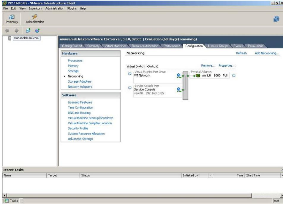
Figure 41: VMware ESX Networking Configuration Screen
