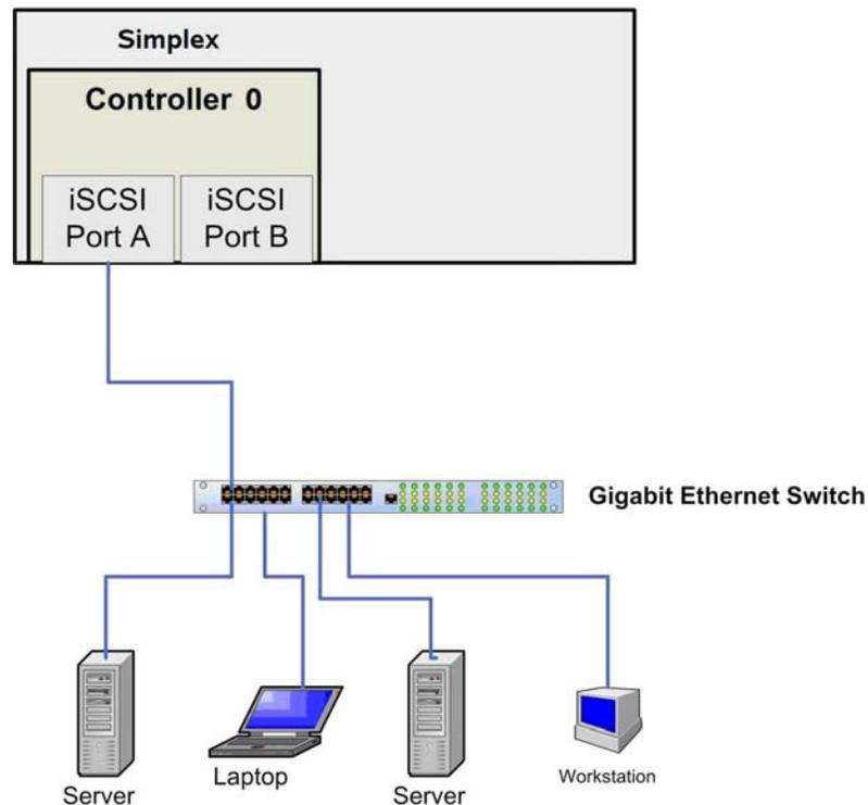
*Figure 6: Non-redundant IP SAN implementation*
