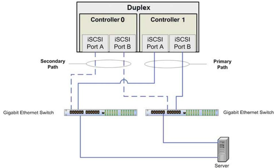
Figure 38: VMware fully redundant iSCSI SAN configuration
