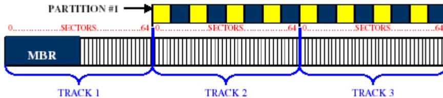
Figure 95: View of a properly Aligned Partition Created with disk drivepart
