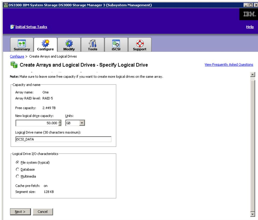
Figure 32: DS3000 Storage Manager Logical Drive Configuration Screen Part2
