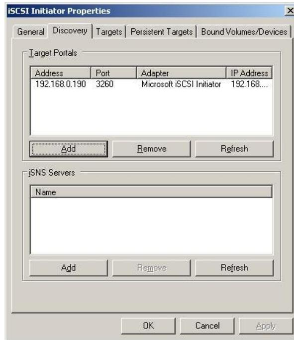
Figure 17: Add the first port of Controller 0 to the target portals.
