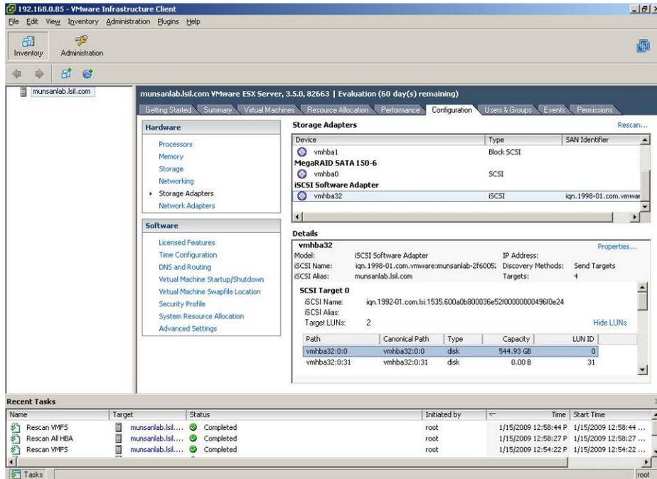
Figure 62: Storage Adapter Configuration Window
