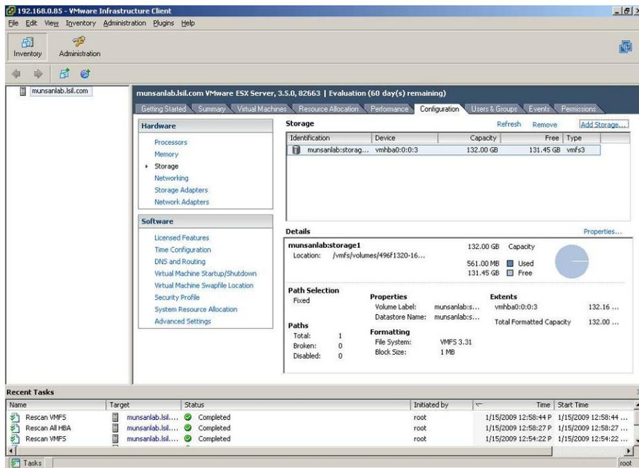
Figure 63: Storage Configuration Tab
