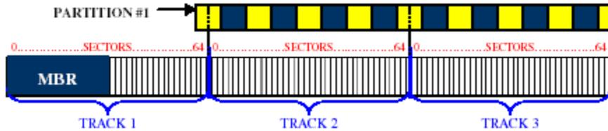
Figure 94: View of a Misaligned Partition that was not created with disk drivepart
