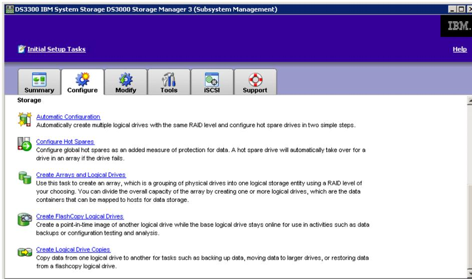
Figure 31: DS3000 Storage Manager Create Arrays and Logical Drives Configuration Screen Part 1
